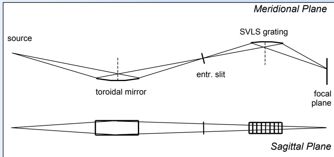
Spherical VLS (SVLS) grating with a toroidal mirror that corrects for the astigmatism
