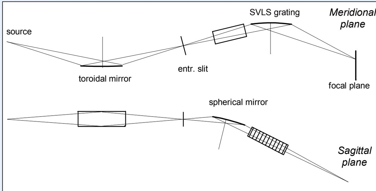
The spherical mirror is mounted with its tangential plane coinciding with the grating equatorial plane
