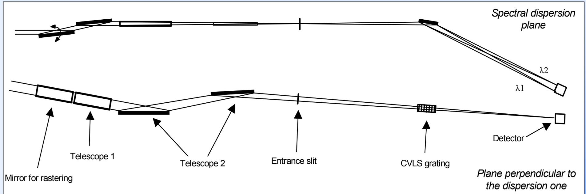
The image within the field-of-view in the direction parallel to the slit has **constant spectral resolution** and **slightly degrading spatial resolution**
